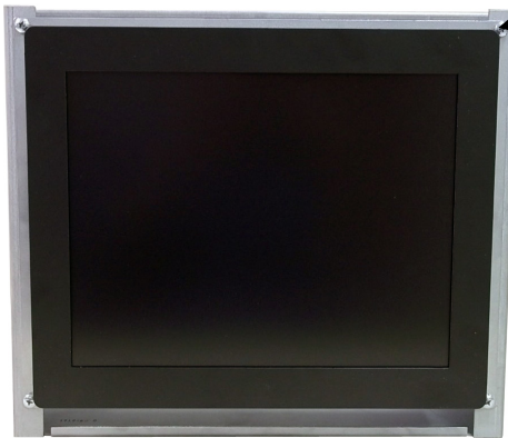
Mount Flat Panel Monitor to Chassis using screws from CRT
